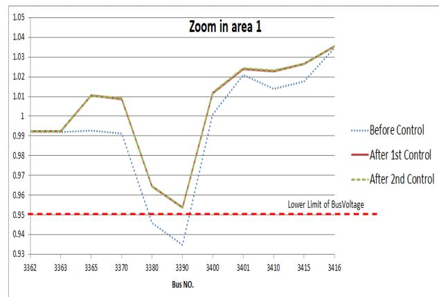
**Fig. 5, Voltage profile in area 1**
