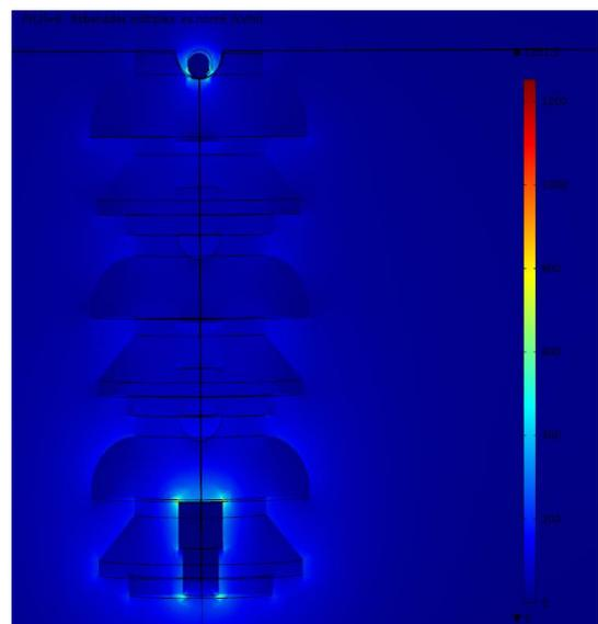
Fig. 18 Distribution of electric field for the chain of insulators with wet surface.
