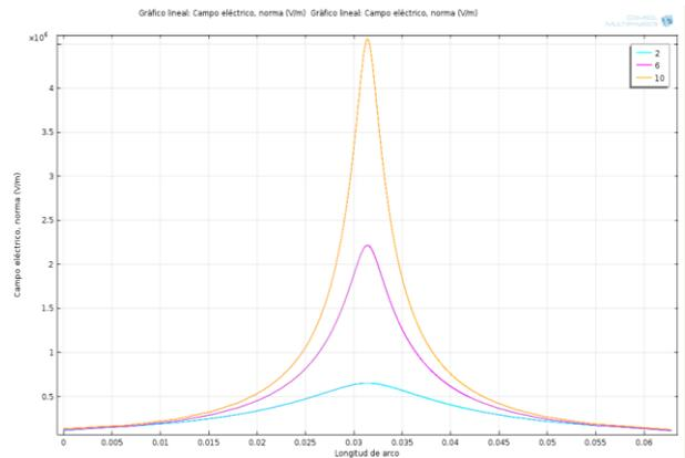
Fig. 12 Electrical field in length of arc for different materials
