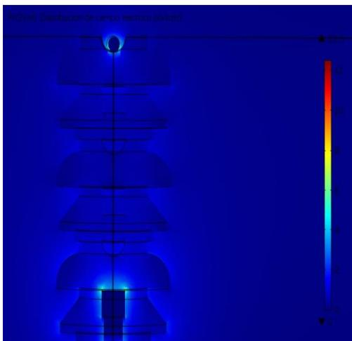
Fig. 5 Electric field distribution in porcelain insulator
