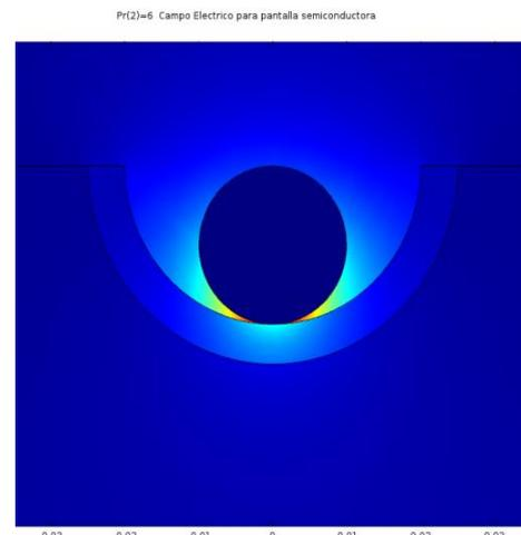
Fig. 13 Level surface of Electrical field in length of arc for different materials with semiconductor plate.
