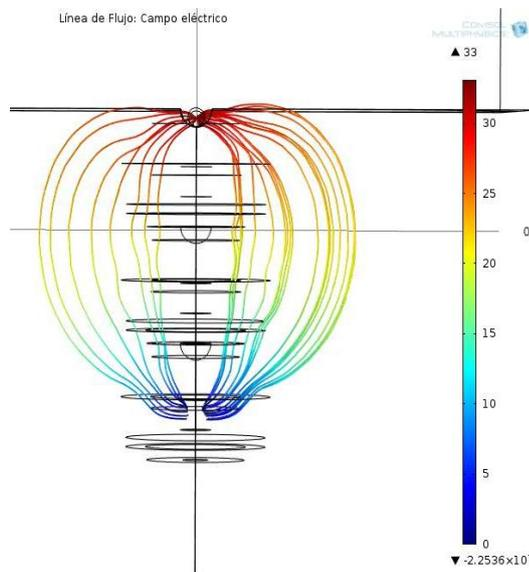
Fig. 10 Lines of flux of electric field in ethyl propylene insulator
