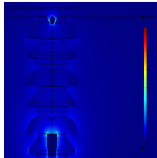
Fig. 7 Distribution of electric field in insulator of ethyl propylene.
