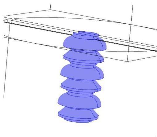
Fig. 3: b) Geometry imported in COMSOL.
