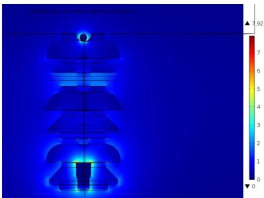
Fig. 16 Electric field distribution for damaged string insulator
