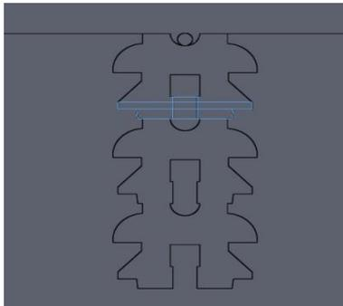
Fig. 15 Level surface of Electric field distribution for damaged string insulator
