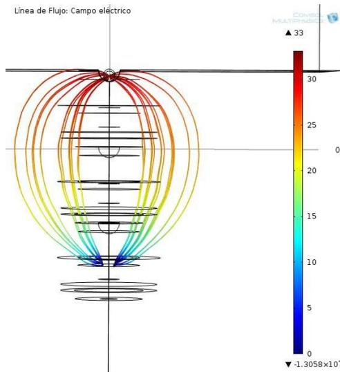
Fig. 9 Flow lines of electric field in porcelain insulator.
