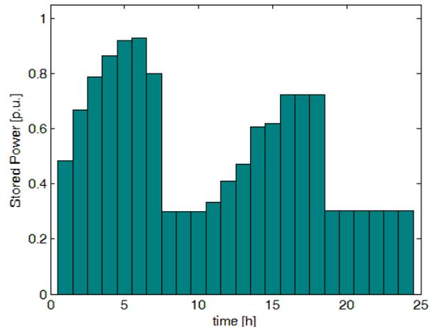
Fig.5. BESS charge level
