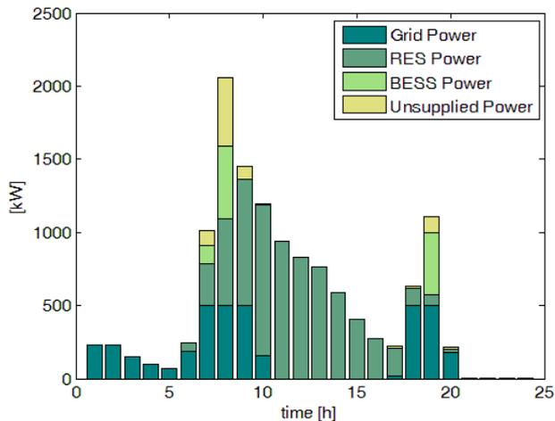
Fig.3. Grid, RES and BESS supplied power
