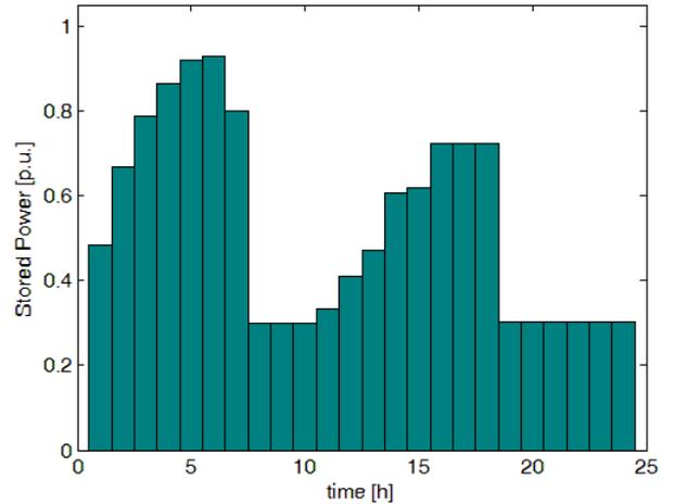
Fig.5. BESS charge level
