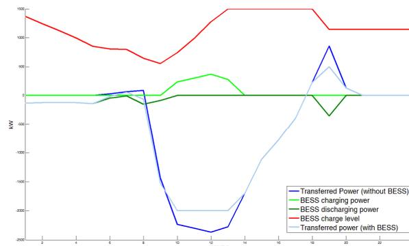
Fig. 2. Power flows from upstream to downstream network
