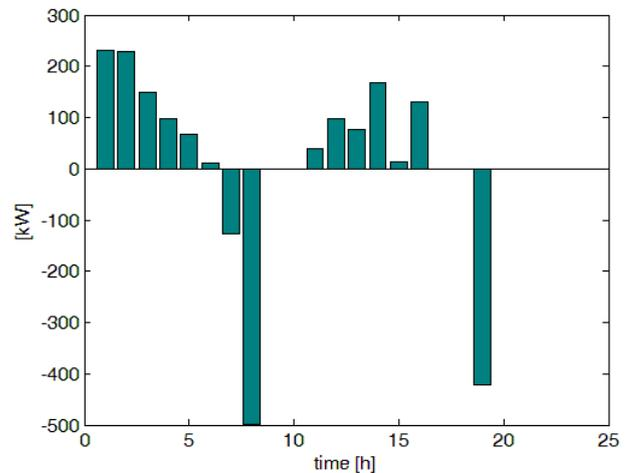
Fig. 6. BESS Charge/Discharge Power
