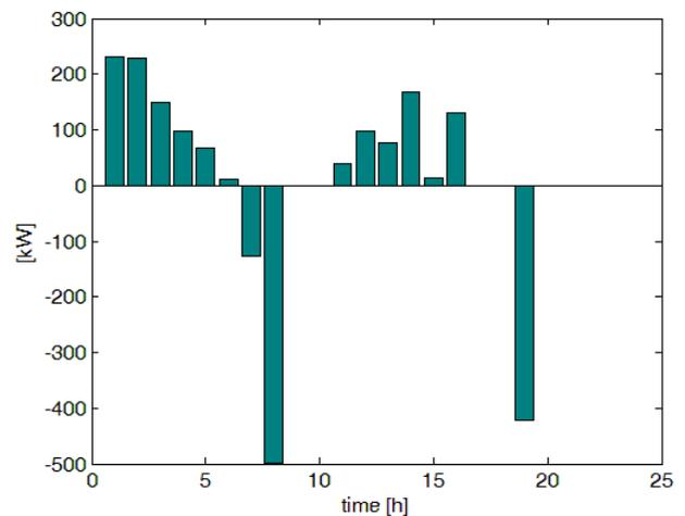
Fig. 6. BESS Charge/Discharge Power
