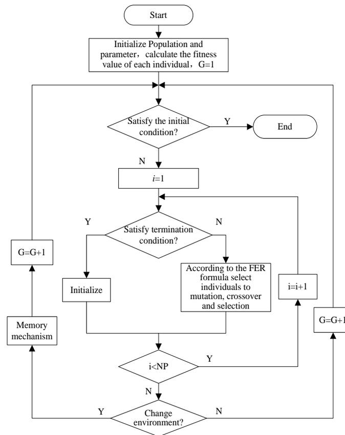
**Figure 1.** The step of Different Evolution Algorithm FER
