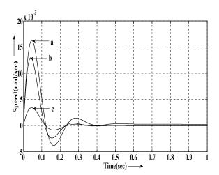
a.Control signal  $\alpha_2$  b. Control signal  $\alpha_2$  and POD c. Control signal  $\alpha_2$  with MFFN Fig.9.Time Domain Analysis of the signal  $\alpha_2$
