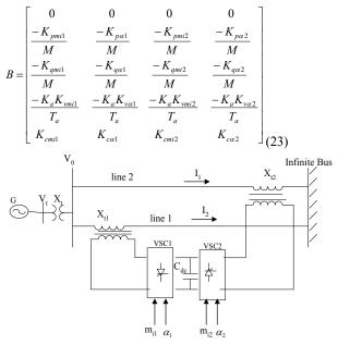
Fig. 1: A single machine infinite bus power system installed with an IPFC in one of the lines
