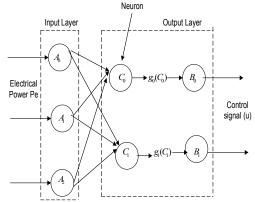
Fig. 4: Structure of MFFN Controller
