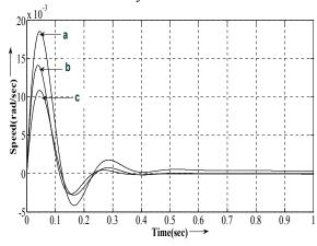
a.Control signal  $\alpha_1$  b. Control signal  $\alpha_1$  and POD c. Control signal  $\alpha_1$  with MFFN Fig.8 Time Domain Analysis of the signal  $\alpha_1$
