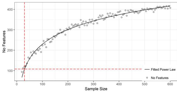
Figure 7: The Random Forest number of relevant features versus training sample size: results and fitted power law curve.
