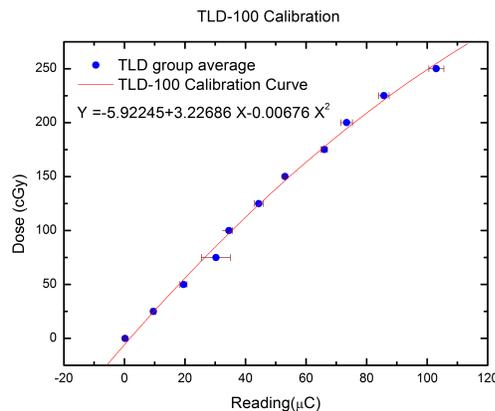
Figure 3: Calibration curve of TLD-100.
