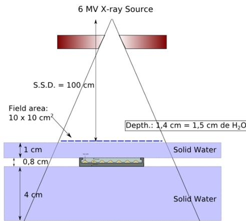
Figure 1: Schematic diagram showing the TLD-100 calibration setup using solid water.
