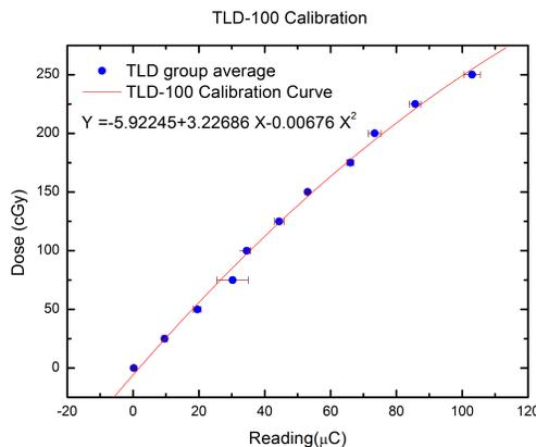
Figure 3: Calibration curve of TLD-100.
