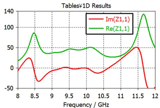
Fig. 8 Frequency characteristics of input impedance.
