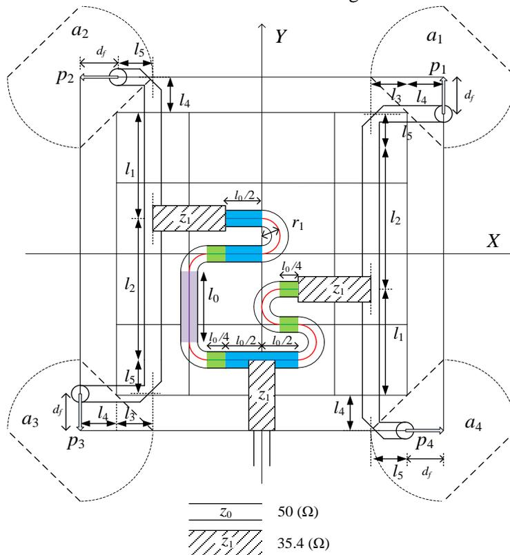
Fig. 5 Configuration of routing wire for feeding.
