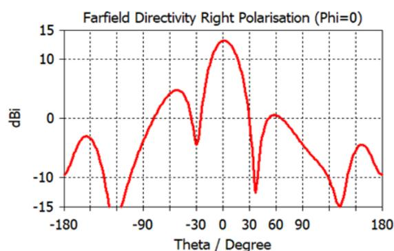
Fig. 10 Radiation pattern at  $\Psi = 0$  (rad) by linear scale.
