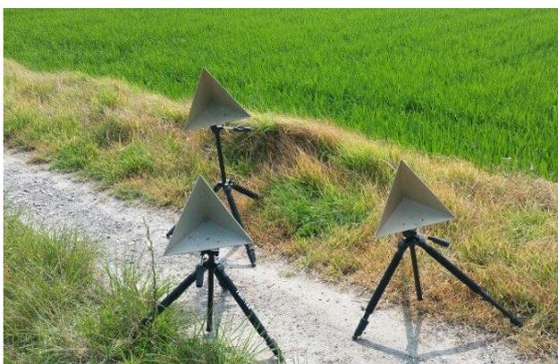
Fig. 7. Corner reflectors.
