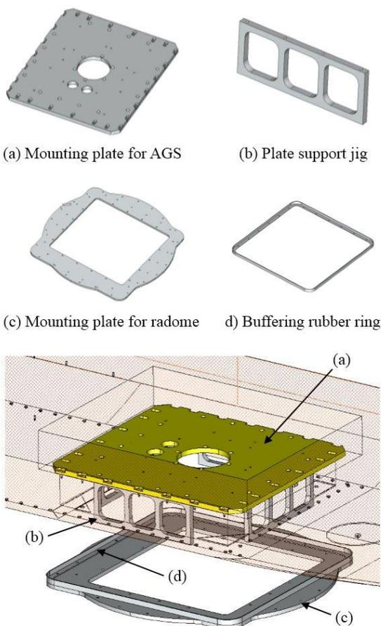
Fig. 2. Jig to install the antenna and gimbal set.
