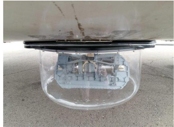
Fig. 3. The AGS installed to PA31-350 aircraft.
