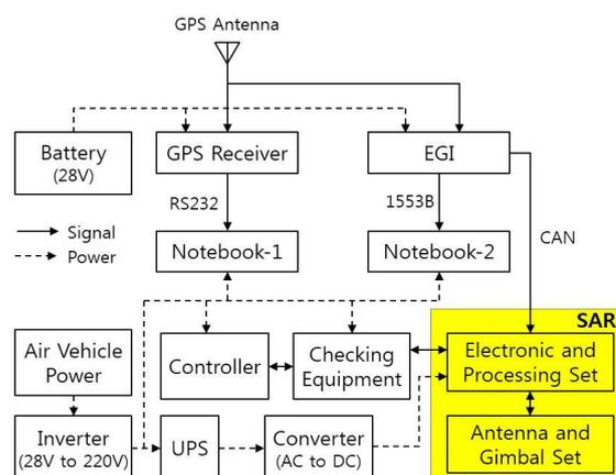
Fig. 1. Block diagram of the SAR testbed.
