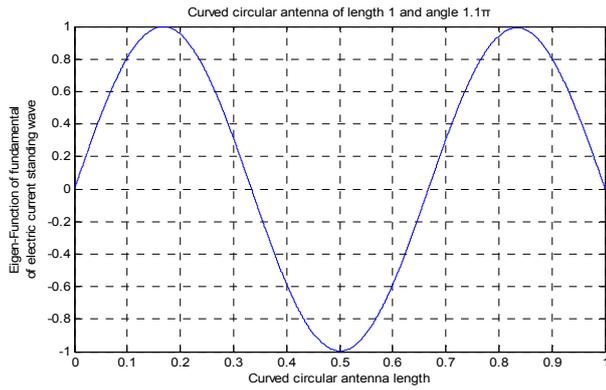
**4. Fundamental standing wave on a circular arc antenna of angle  $1.1\pi$**
