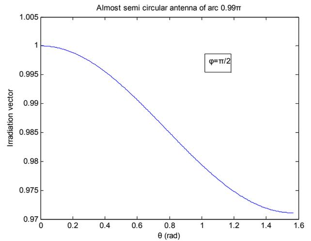
**Fig 7. Radiation for variable  $\theta$  and  $\phi=\pi/2$**
