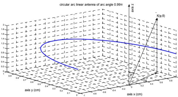
**Fig 5. A linear circular arc antenna of arc angle  $0.99\pi$**
