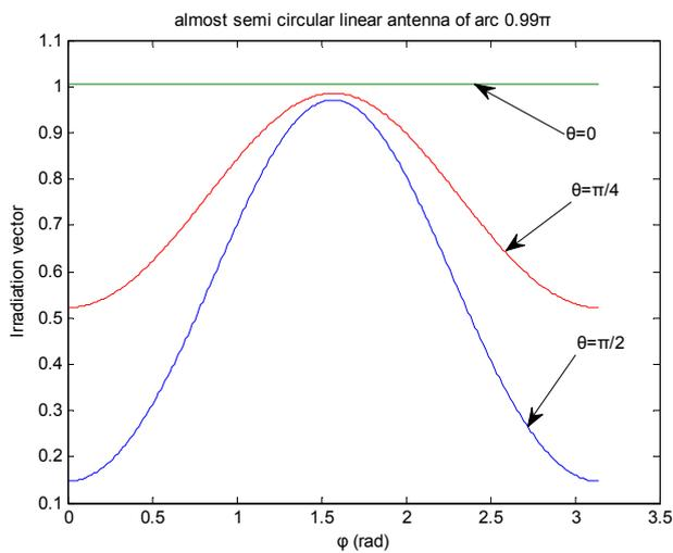
**Fig 6. Radiation for variable  $\phi$  and  $\theta=\pi/2, \pi/4, 0$**
