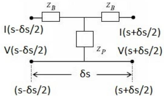
**Fig. 1** Schematic diagram of the representative T-circuit.
