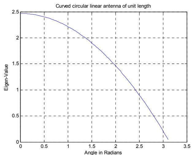
**Fig.2** Fundamental Eigen-value as function of the arc angle in radians of a circular arc antenna.
