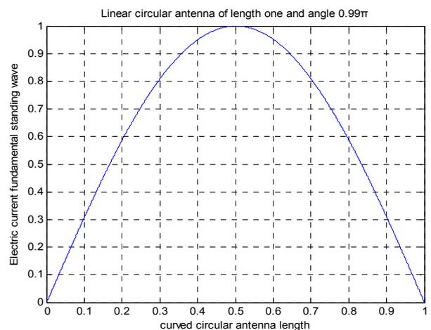
**Fig 3.** Fundamental standing wave on a circular arc antenna of angle  $0.99\pi$
