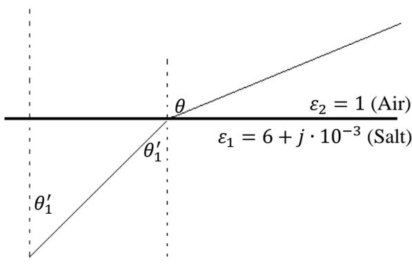
Fig.3 Transmission of the ray from salt to air
