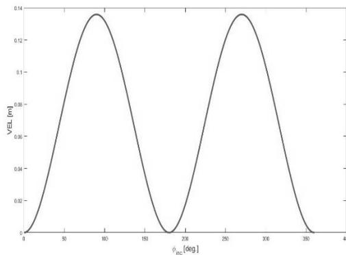
Fig.5 Vector Effective Length plotted versus  $\phi_{inc}$  angle
