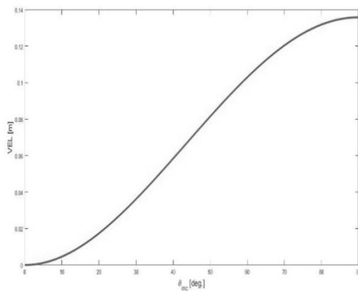
Fig.4 Vector Effective Length plotted versus  $\theta_{inc}$  angle
