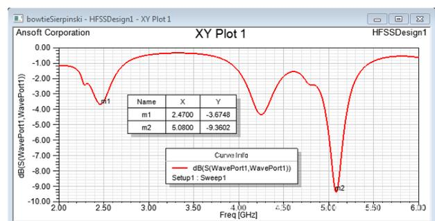
Fig. 3. Return loss for the fractal bowtie antenna without CSRR.
