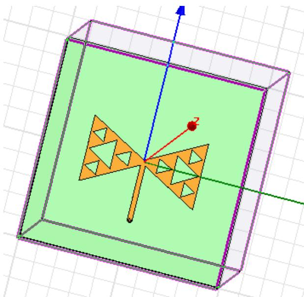
**Fig. 6.** Front side of the fractal bowtie antenna with CSRR.
