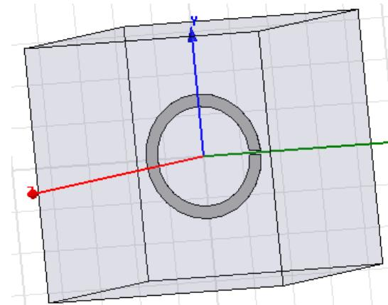
Fig. 4. Circular Split Ring Resonator.
