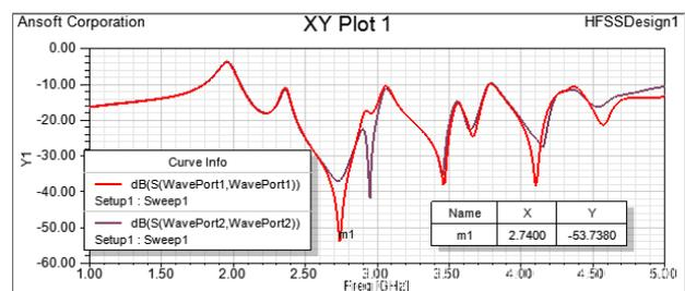
Fig. 5. Return losses for the circular split ring resonator.
