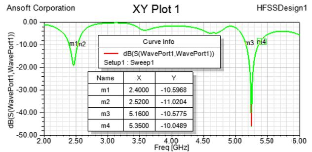
Fig. 8. Return losses for the fractal bowtie antenna with CSRR.
