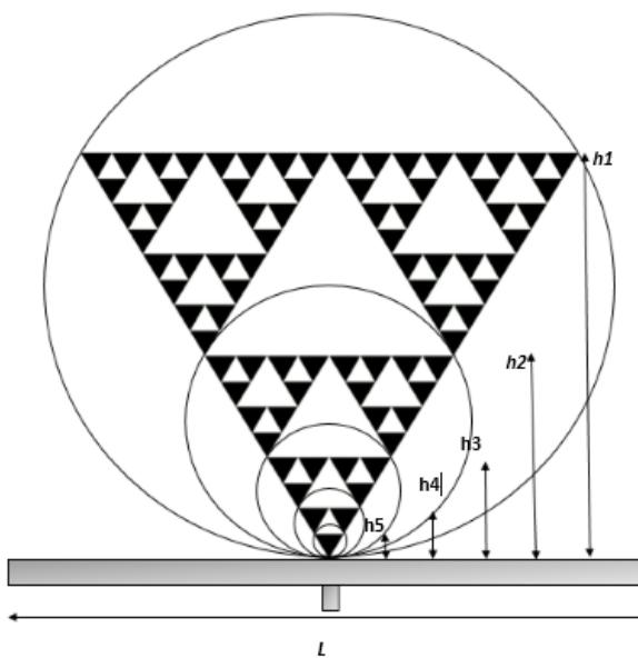
**Fig. 1.** Sierpinski fractal geometry of five iterations.
