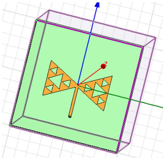
Fig. 6. Front side of the fractal bowtie antenna with CSRR.
