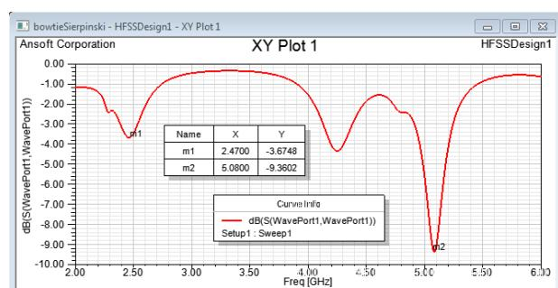
Fig. 3. Return loss for the fractal bowtie antenna without CSRR.
