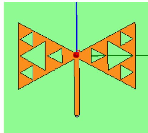
Fig. 2. Fractal microstrip bowtie antenna with  $\lambda/4$  transmission line feeder.
