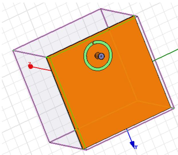
Fig. 7. Back side of the fractal bowtie antenna with CSRR..
