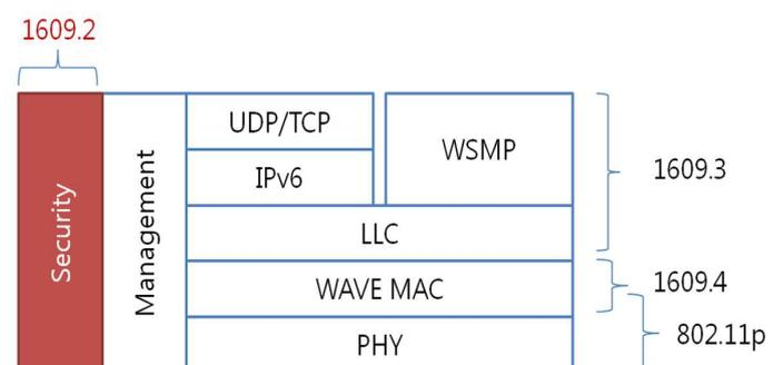
Fig. 1. WAVE reference model.
