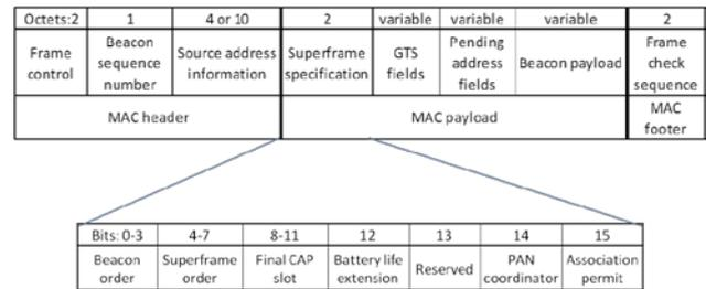
Fig. 3. Structure of the Beacon frame
