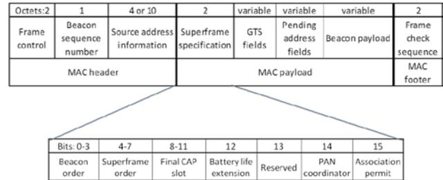
Fig. 3. Structure of the Beacon frame
