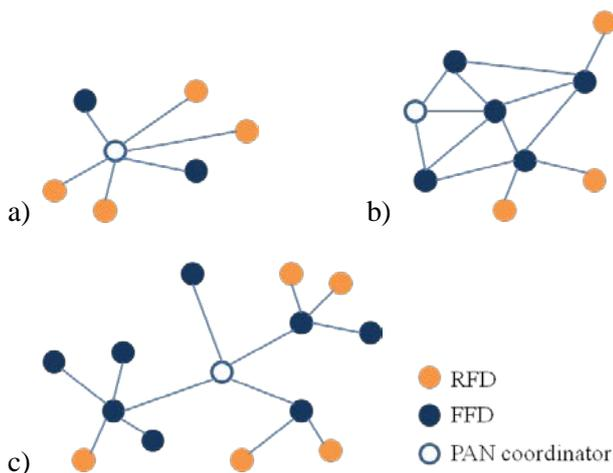
Fig. 1. Network topologies: a) star, b) mesh, c) cluster-tree.
