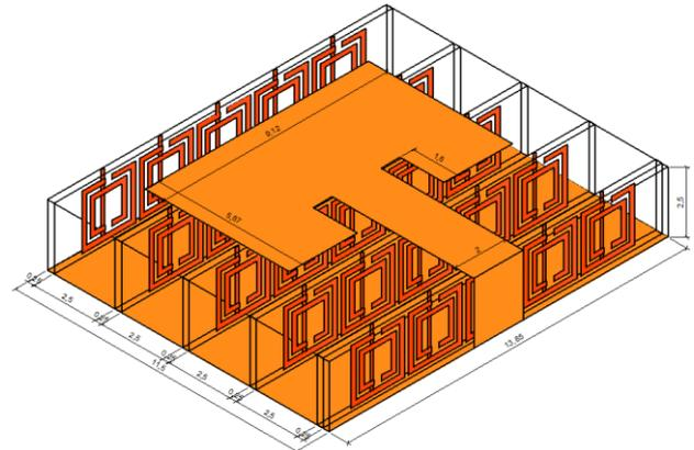
Fig. 5 - Microstrip antenna dimensions with metamaterial substrate.
