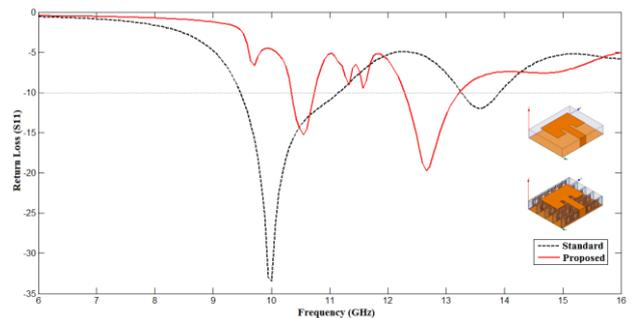
Fig. 6 - Comparison of return loss between the pattern microstrip antenna and the one with metamaterial substrate.
