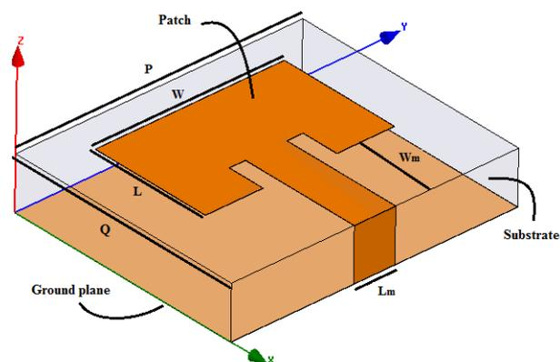
Fig. 1 - Microstrip antenna pattern to 10 GHz.
