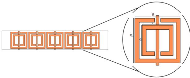
Fig. 3 - Substrate Structure with SRR.
