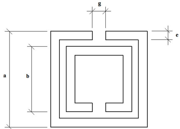
Fig. 2 – Dimensions of physical geometry of SRR.
