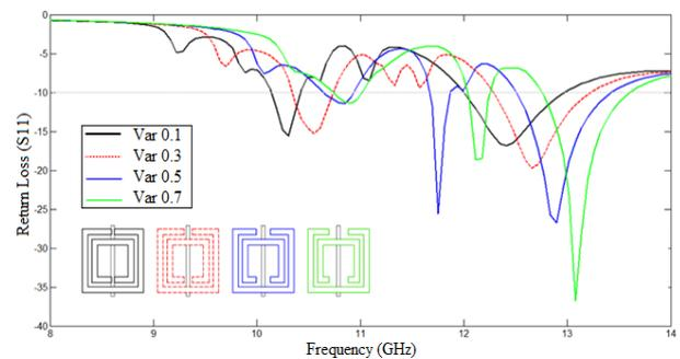
Fig. 8 - Return loss response for the ring gap variations.
