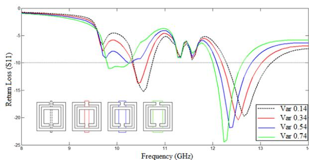
Fig. 7 - Return loss response for the thick wire variation.
