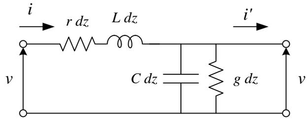
Fig. 2 Equivalent circuit of unmyelinated axon of length  $dz$  with loss.
