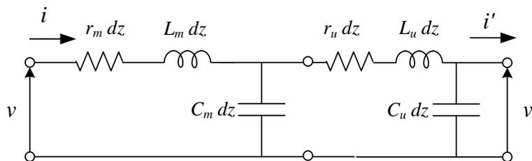
Fig. 4 Equivalent circuit of axon with myelinated and unmyelinated parts.  $L_m, C_m,$  and  $L_u, C_u$  are circuit parameters corresponding to myelinated and unmyelinated parts of an axon.
