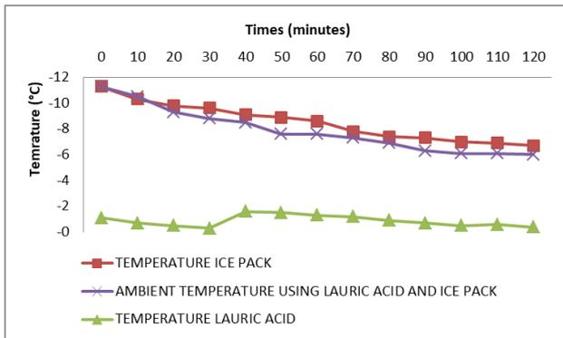
Figure 9. Cooler box graph using 250 gram lauric acid and ice pack as control
