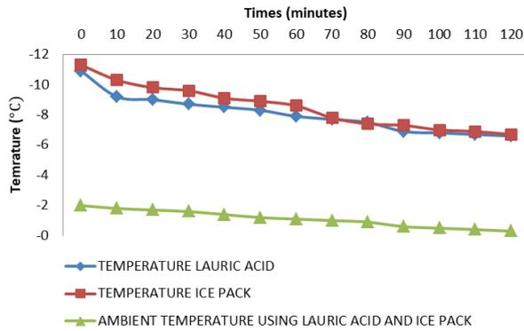
Figure 11. Cooler box graph using 150 gram lauric acid and ice pack as control
