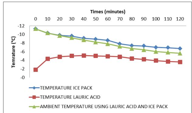
Figure 12. Cooler box graph using 100 gram lauric acid and ice pack as a control
