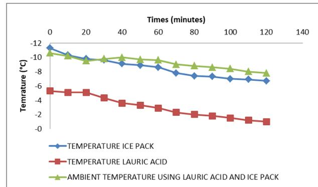
Figure 10. Cooler box graph using 200 gram lauric acid and ice pack as control
