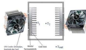
Figure 3. Heatsink on the hot side and cold side.
