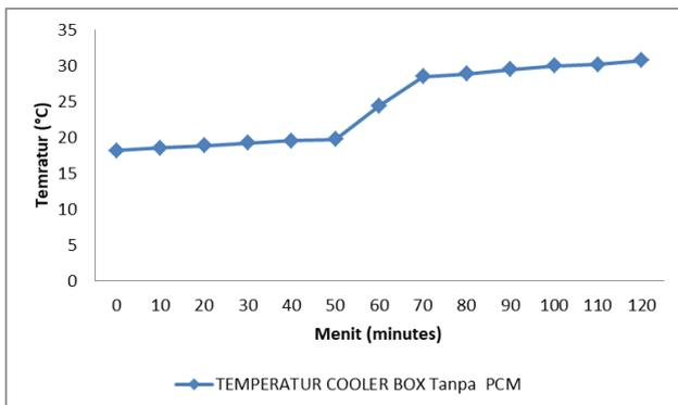
Figure 7. Cooler box graph without PCM.
