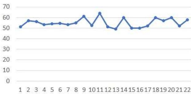
Figure 3 Graph. Hardness Value of ST37 Steel Before Heat Treatment
