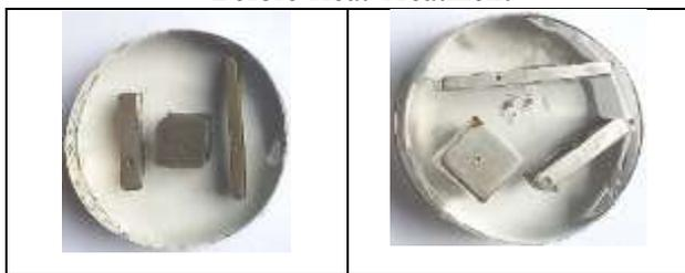
Figure 4.A ST37 Steel Specimen
