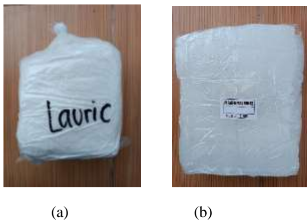
Fig. 2. PCM used (a). lauric acid, (b). paraffin wax
