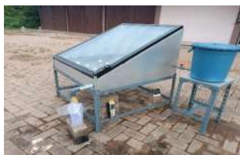
Fig. 1. Solar desalination device with PCM
