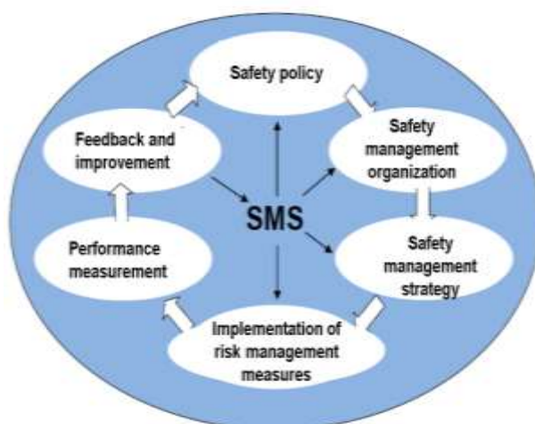
Fig. 7. Tasks specified in the safety management system (SMS) of technical installation with SMR.
