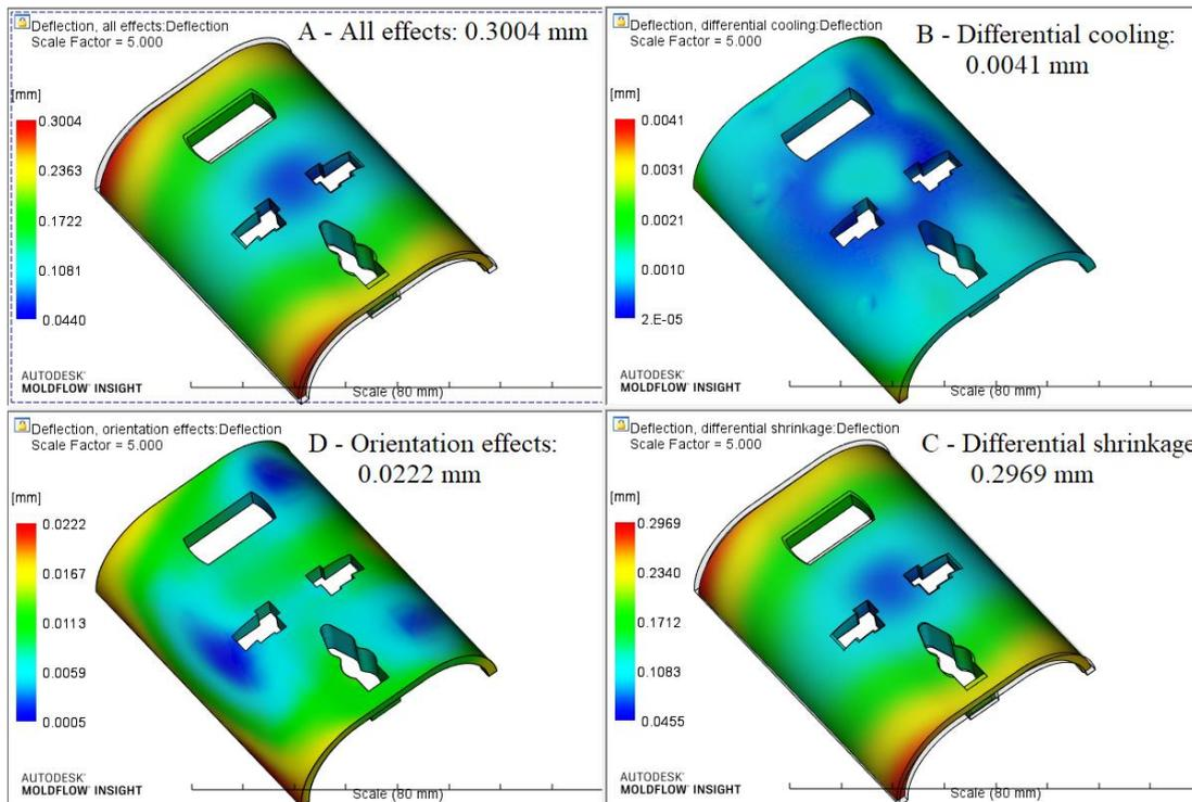
Fig. 8: Investigation of causes of warpage with initial study
