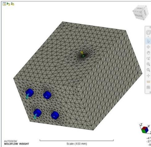
Fig. 5: Meshed Mould Volume with Cooling and Feed System
