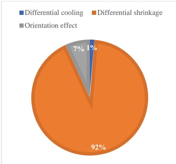
Fig. 9: Causes of Warpage – Initial Study
