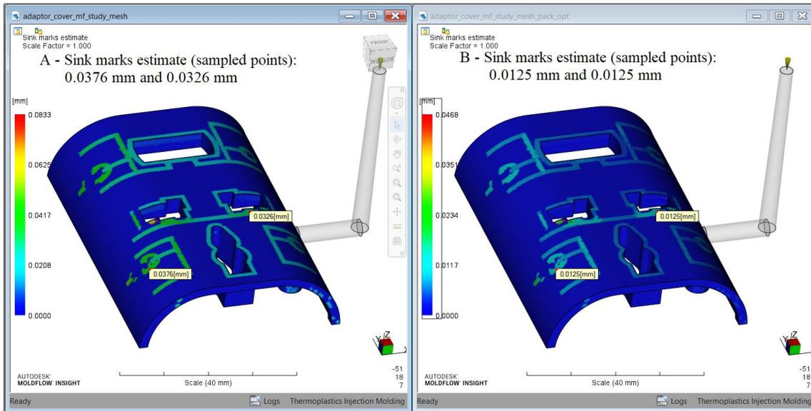
Fig. 7: Comparison of Sink Marks Estimate with default Packing Profile (left) and Optimised Packing Profile (right)
