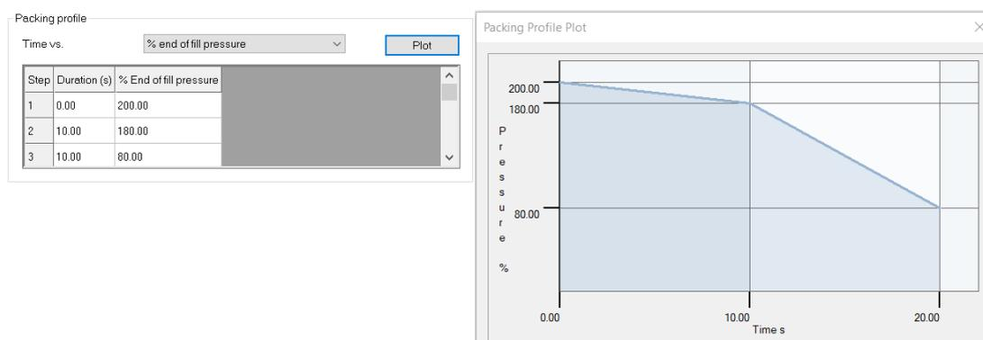
Fig 4: Optimised Packing Profile and Plot for desirable Volumetric Shrinkage
