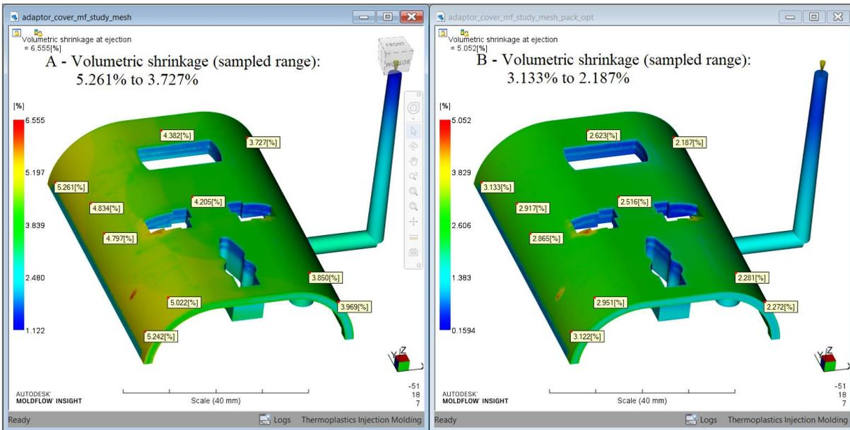
Fig. 6: Result of Volumetric Shrinkage at Ejection with default Packing Profile (left) and Optimised Packing Profile (right)
