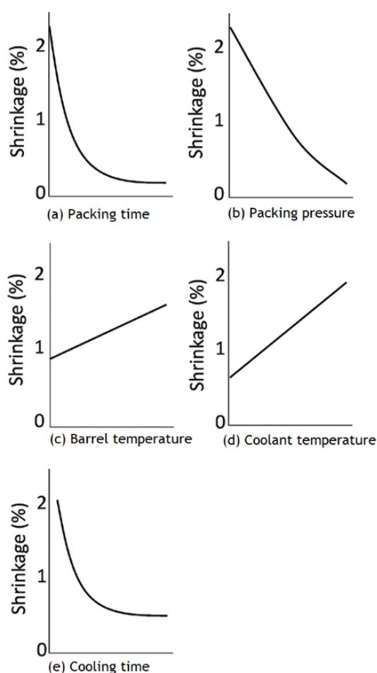
Fig. 1: Effect of processing conditions on shrinkage [4]
