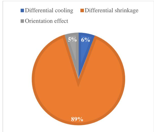
Fig. 10: Causes of Warpage - Optimised Study
