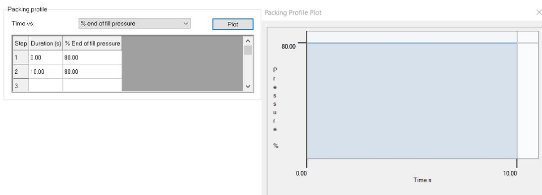
Fig 3: Initial Packing Profile and Plot
