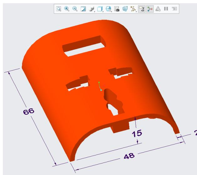
Fig 2: Three-Dimensional Model of Electric Socket Adaptor
