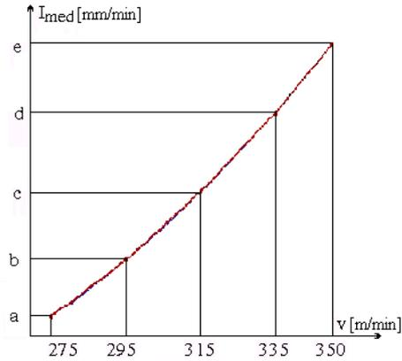
Figure 14 Variation of the average wear rate with the cutting speed
