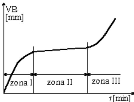
Figure 3 The evolution of wear over time
