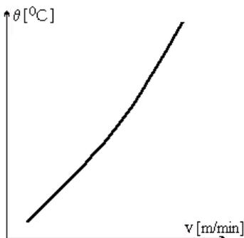
Figure 13 Temperature variation with cutting speed
