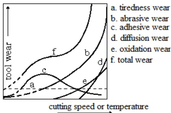
Figure 1. The influences of partial wear on total wear
