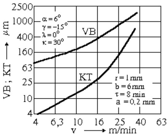
Figure 8 Variation of the characteristic dimensions of the wears depending on the cutting speed
