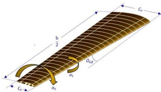
Fig 1. Geometric Properties for subsonic wing of aircraft
