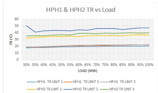
Figure 5.11 HPH1 and HPH2 TR vs Load Trend
