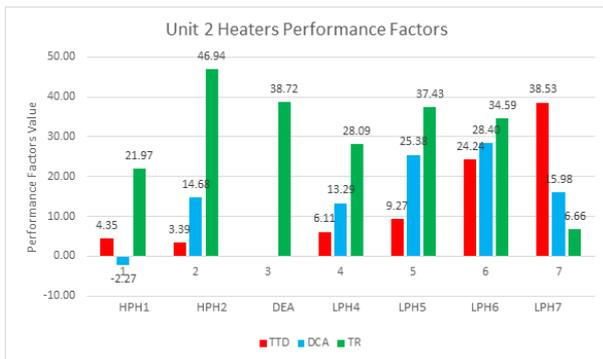
Figure 5.3 Unit 2 Performance Result 135 MW
