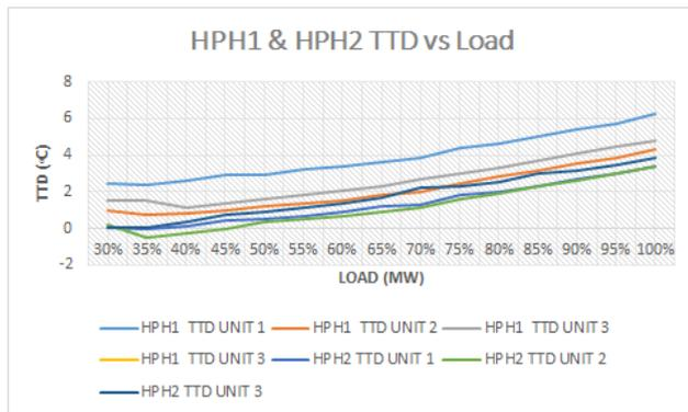
Figure 5.5 HPH1 and HPH2 TTD vs Load Trend
