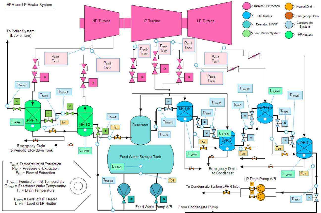
Figure 3.1 Experiment System Set-up Process Flow with instrument locations
