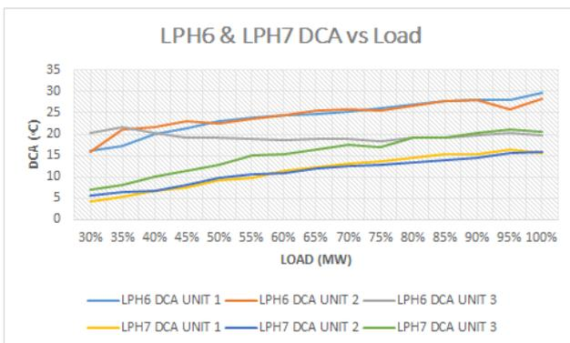
Figure 5.10 LPH6 and LPH7 DCA vs Load Trend
