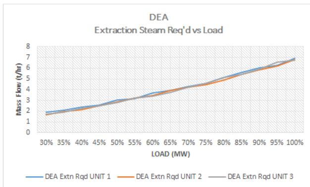
Figure 5.16 DEA Extraction Steam Flow Required
