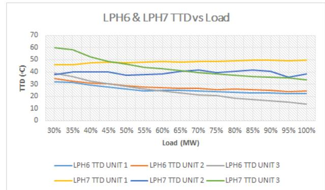
Figure 5.7 LPH6 and LPH7 TTD vs Load Trend
