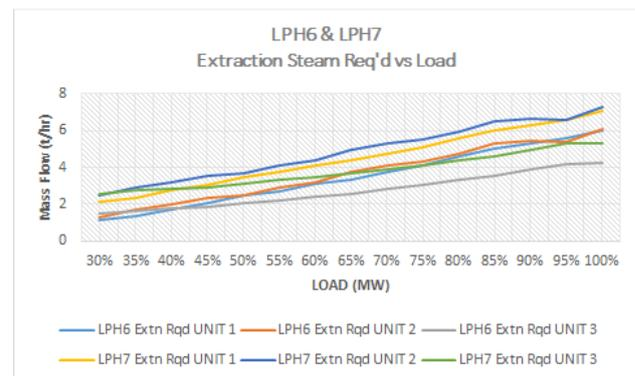
Figure 5.18 LPH6 & LPH7 Extraction Steam Flow Required
