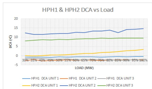
Figure 5.8 HPH1 and HPH2 DCA vs Load Trend
