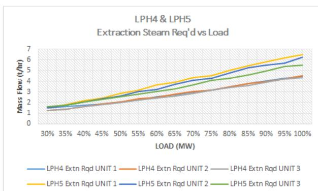
Figure 5.17 LPH4 & LPH5 Extraction Steam Flow Required
