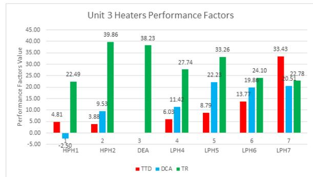
Figure 5.4 Unit 3 Performance Result 135 MW
