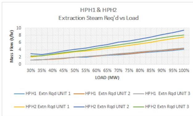
Figure 5.15 HPH1 & HPH2 Extraction Steam Flow Required
