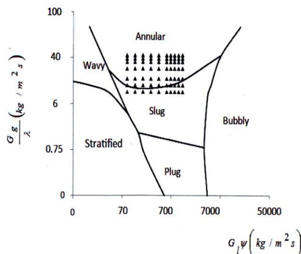
Fig. 3 Flow pattern prediction by Baker flow pattern map [5]
