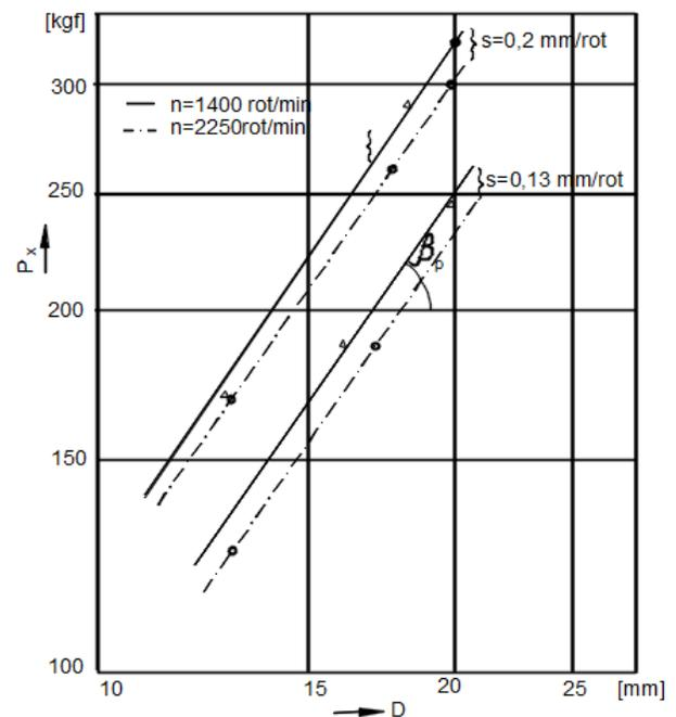
Fig.5 Variation of axial force depending on the drill diameter.
