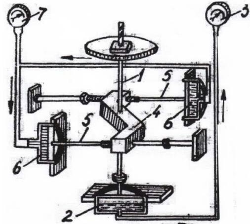
Fig.2 The schematic diagram of a hydraulic dynamometer.
