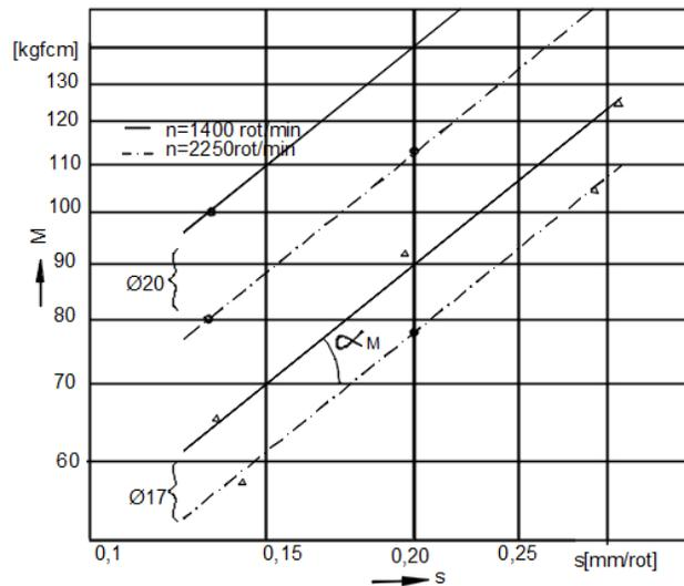
Fig.4 Variation of the torque depending on the drill feed.
