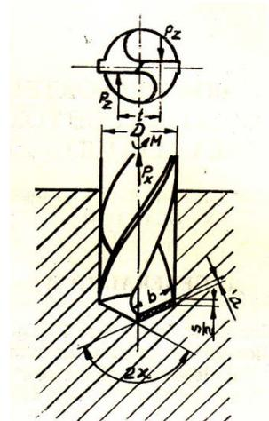
Fig.1 Axial force and torque at drilling operation.
