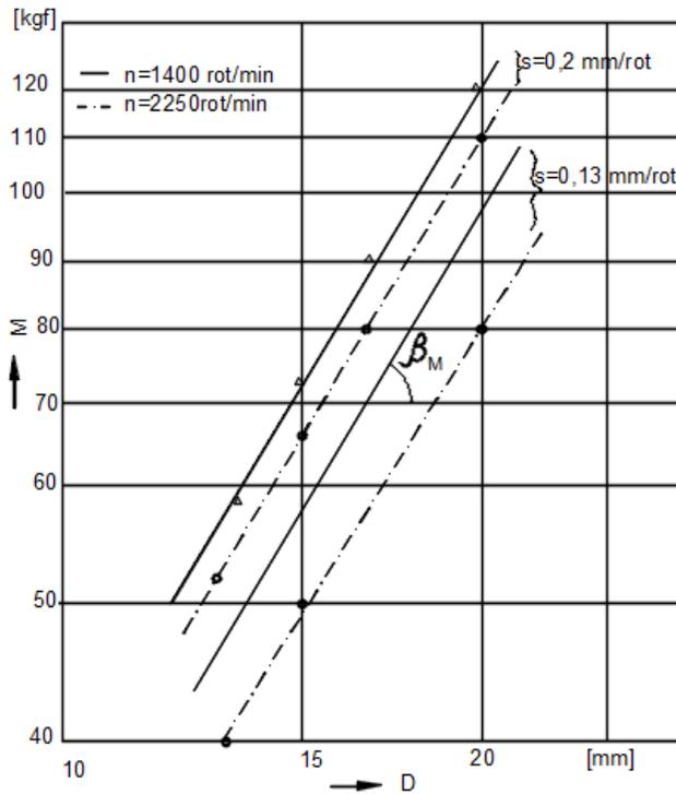
Fig.6 Variation of the torque depending on the drill diameter.
