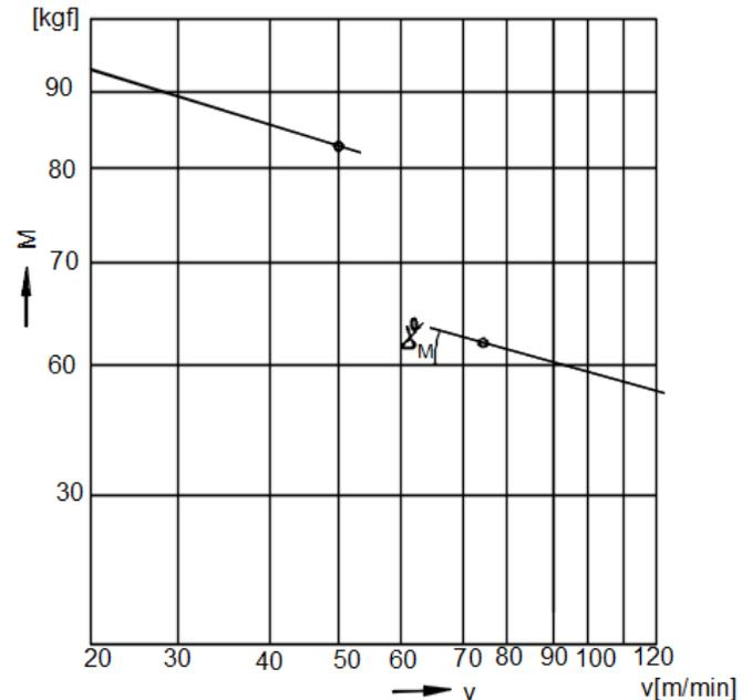
Fig.8 Variation of the torque depending on the cutting speed.
