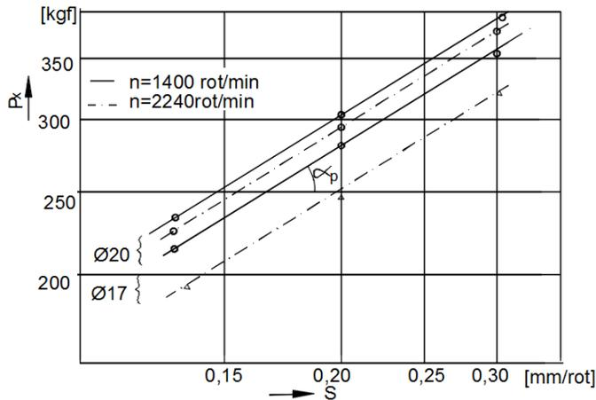
Fig.3 Variation of axial force depending on the drill feed.
