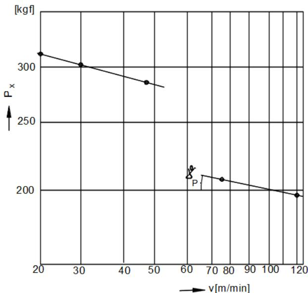
Fig.7 Variation of the axial force depending on the cutting speed.
