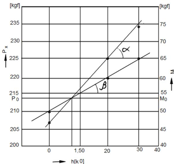
Fig.9 Variation of the axial force depending on the depth of the hole.
