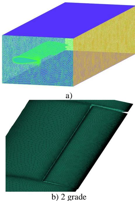
Fig.3 Grid for the computational domain: a) entire domain, b) aileron at 2°
