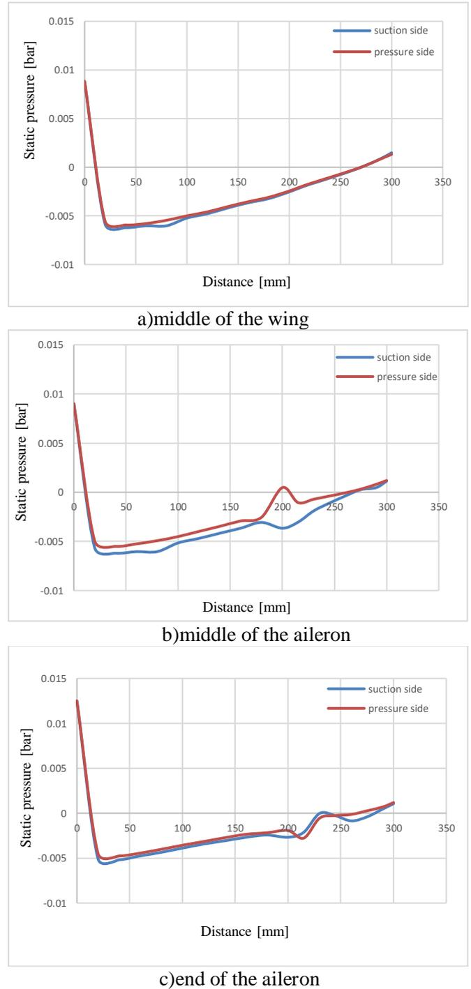
Fig.6 Pressure Distribution relative to the distance from the leading edge
