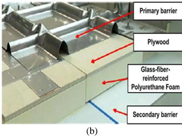
**Fig. 1** (a) Schematic and (b) photograph of the liquefied natural gas insulation system
