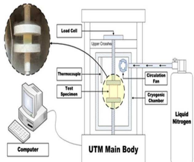
**Fig. 3** Schematic diagram of the experimental apparatus for the low-temperature compression test
