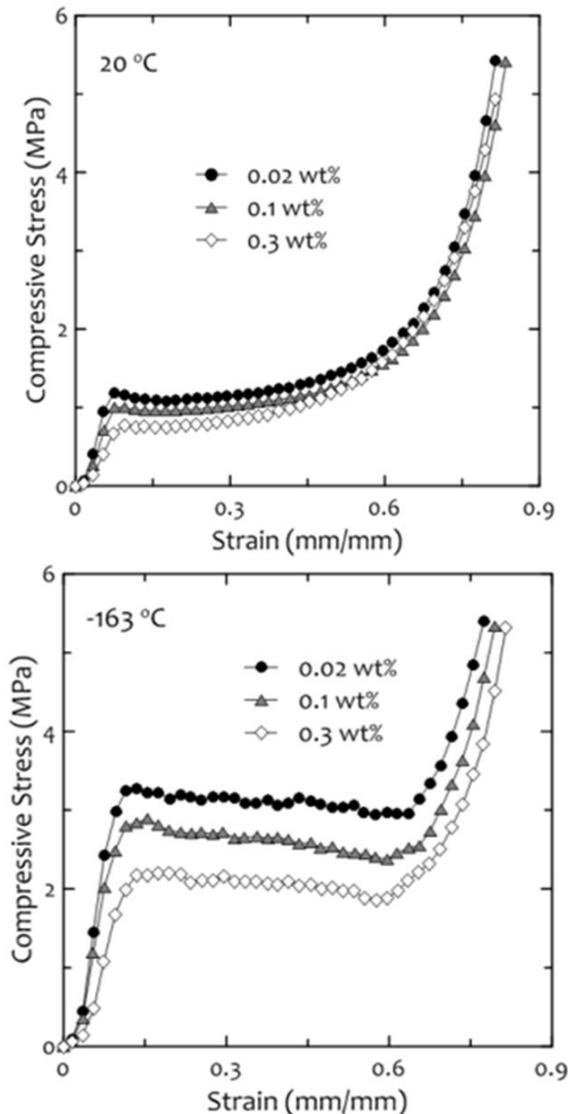
**Fig.4** Temperature dependent compression test result of carbon nanotube polyurethane foam
