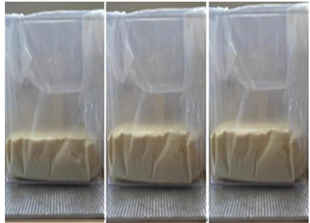
**Fig. 2** Photographs of the foaming process of the polyurethane foam
