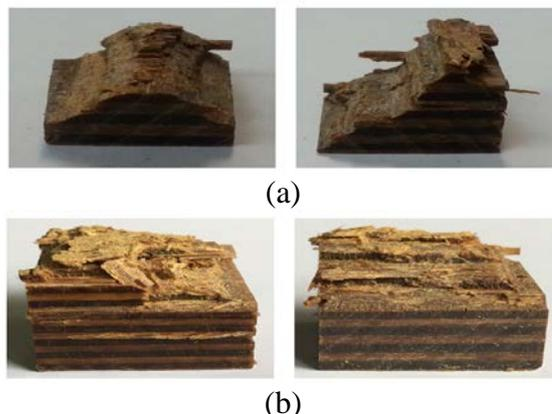
**Fig. 4** Fracture characteristics for the RT samples in the (a) room temperature and the (b) cryogenic tests
