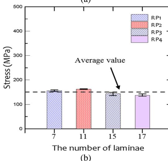
**Fig. 2** Compressive strength of samples under compressive loads in (a) parallel and (b)
