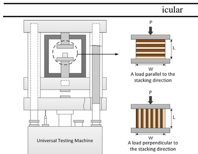
**Fig. 1** Schematic diagram of the universal testing machine and compressive load directions
