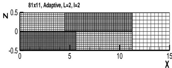
Fig. 1. Block nested grid refinement approach for a short pipe, based grid size:  $81 \times 11$ , two (2) levels of refinement, integer refinement factor equal to two (2).
