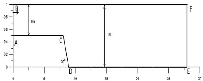
Fig. 2. Geometry description of the inclined step pipe. The dimensionless lengths of the channel vary according to the Re number value.
