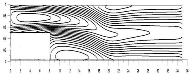
Fig. 8. Velocity contours along the pipe. Block nested grid,  $I=2$ ,  $l=2$ . Inclination angle equal to  $90^\circ$  and  $Re=1200$ . Very clearly are depicted upper and lower wall separation zones.
