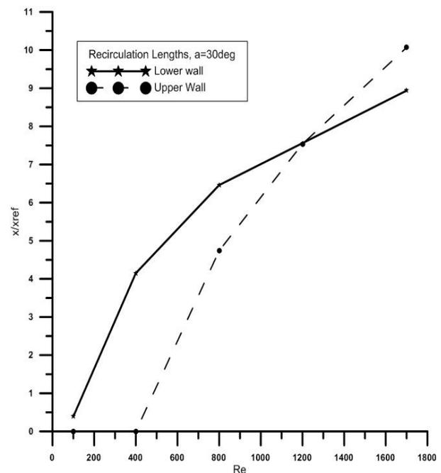
Fig. 4. Recirculation length variation according to the  $Re$  number.
