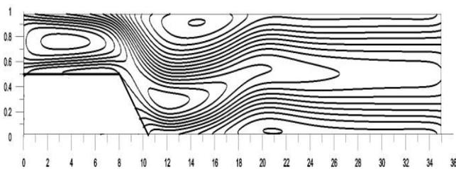
Fig. 6. Velocity contours along the pipe. Block nested grid,  $I=2$ ,  $l=2$ . Inclination angle equal to  $10^\circ$  and  $Re=1200$ . Very clearly are depicted upper and lower wall separation zones.
