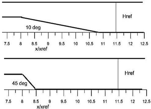
Fig.3. Part of the geometrical physical domains of the incline step pipe for two (2) values of the step angle.
