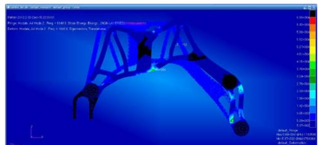
Figure 6: Strain energy (without ROD) – mode 2
