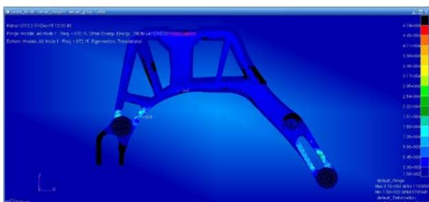
Figure 10: Strain energy (with ROD) – mode 1
