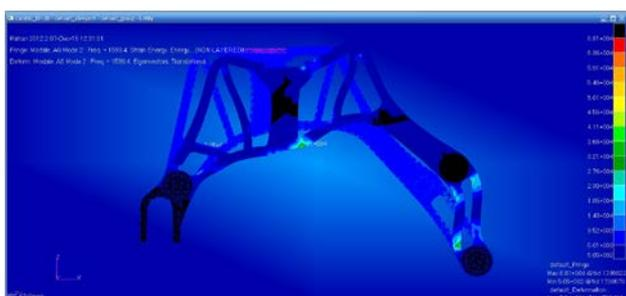
Figure 11: Strain energy (with ROD) – mode 2
