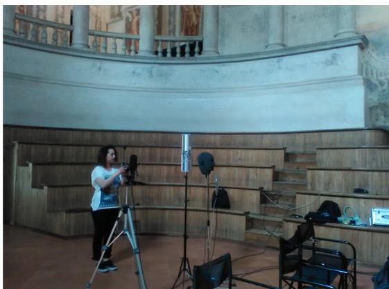
Figure 2 Measurements in the Teatro all'Antica in Sabbioneta, Italy, with the 3D Cylindrical array
