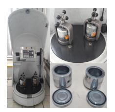
Fig.1. Pulverisette 7 planetary ball mill and vials used in experiment.
