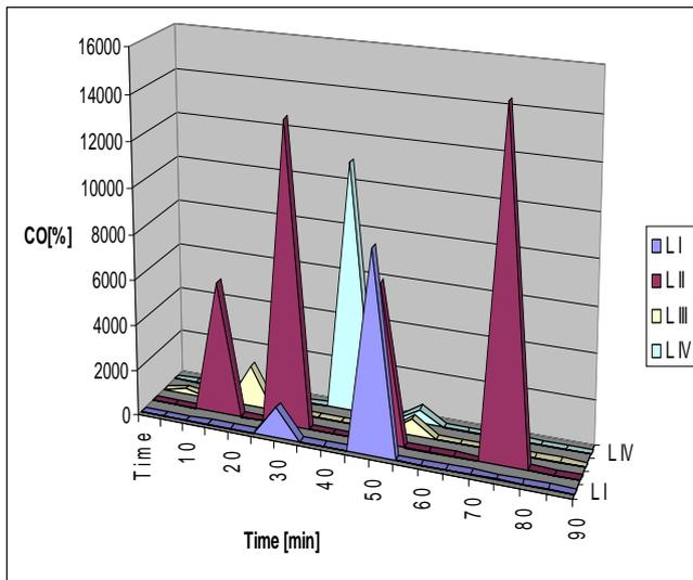
Fig. 7. CO concentration in the evacuated gas during the melting in the EAF
