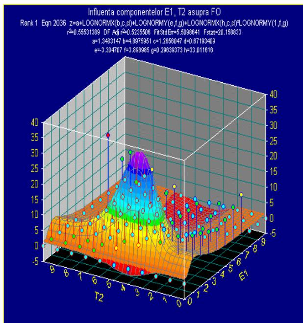
Fig. 11. The cumulated correlation between the criteria function's (CF) prescribed level and  $\bar{T}$  and  $\bar{E}$  vectors' variation.
