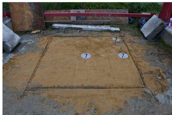
Fig.2 Positions of geotechnical pressure cells
