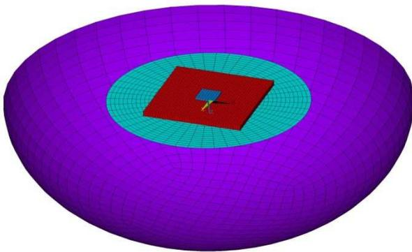
Fig.5 Model of slab resting on the subsoil. Purple semi-infinite elements, cyan solid subsoil elements, red solid plate elements, blue steel plate shell elements.
