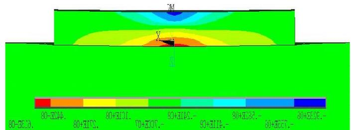
Fig.8 Normal stress sx in the transverse cross-section
