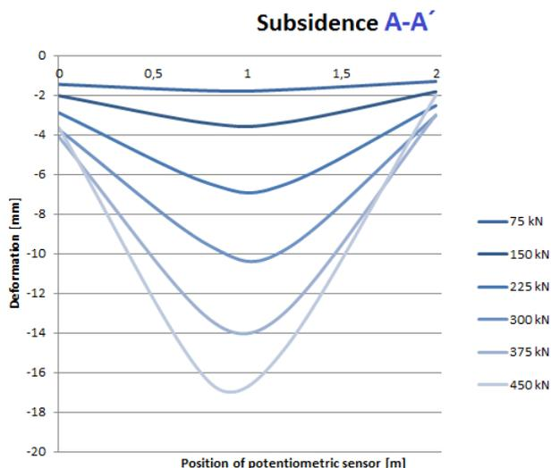
Fig.4 Subsidence line A-A'
