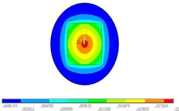
Fig.6 Total vertical displacement of the subsoil model [m]
