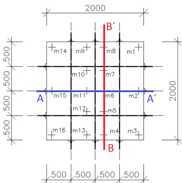
Fig.3 Schematic plan of potentiometers
