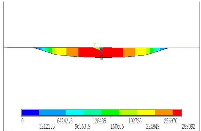
Fig.7 Contact pressure in transverse cross-section
