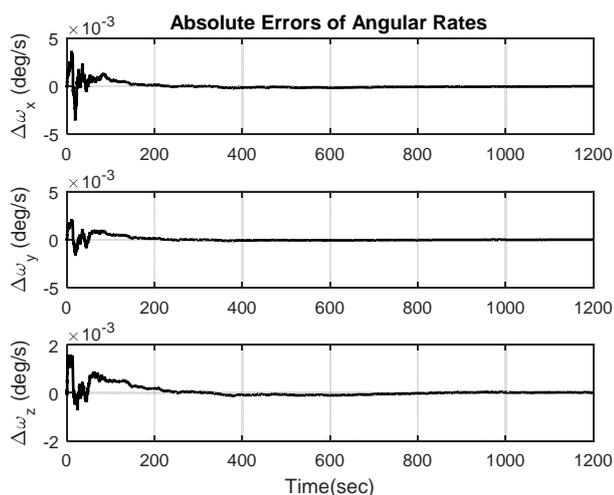
Fig. 6. Angular rate estimation errors of SVD/UKF method.
