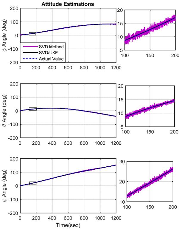
Fig. 2. Attitude estimation of the SVD, and SVD/UKF algorithm with respect to actual simulation values.
