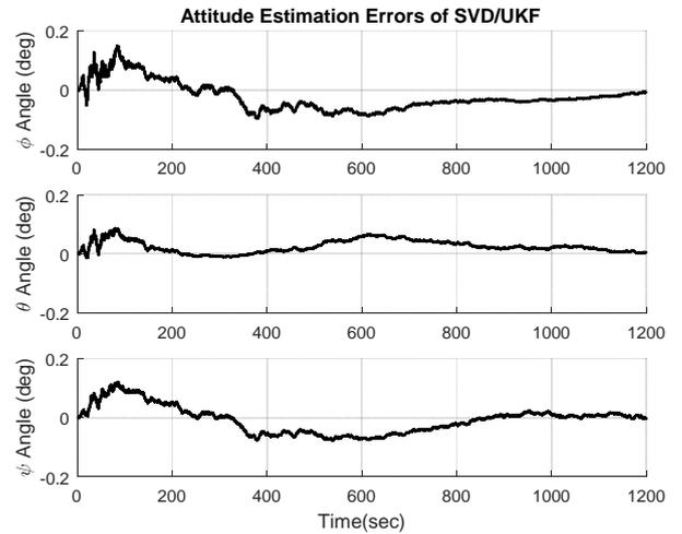
Fig. 4. Attitude estimation errors of SVD/UKF method.
