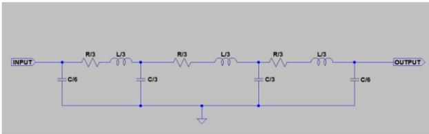
Figure 4. Copper interconnect π-model circuit
