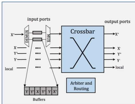
Figure 2. Typical 5-port router
