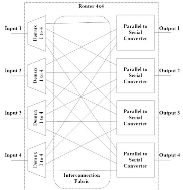
Figure 3. Nanoelectronic router diagram
