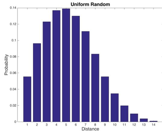
Figure 5. CPD for uniform random traffic pattern in a 8x8 mesh network.
