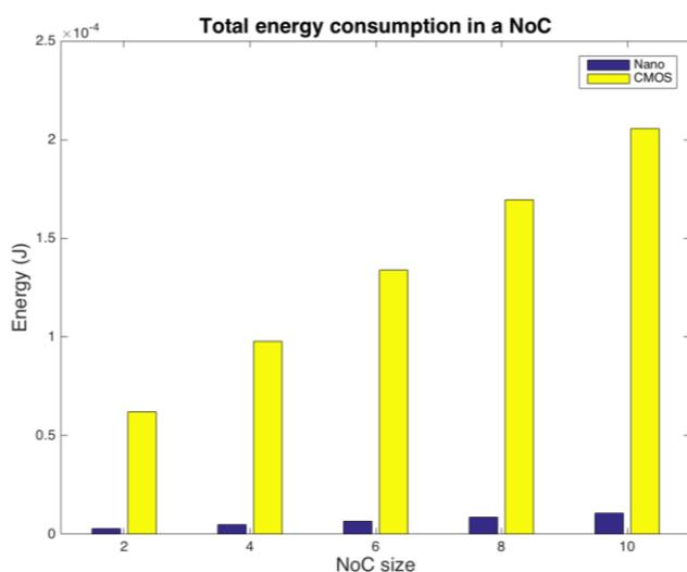
Figure 6. Performance comparison between MOS and nanoelectronic NoCs
