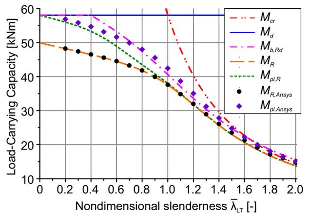
Fig. 7: Resistance vs. non-dimensional slenderness
