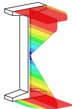
Fig. 12: Course of the von Mises  $\sigma_{vM}$  in the cross-section in the span middle for slenderness  $\bar{\lambda}_{LT} = 0.6$  at reaching the total resistance
