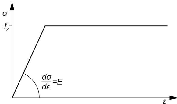
Fig. 6: Bilinear stress-strain diagram
