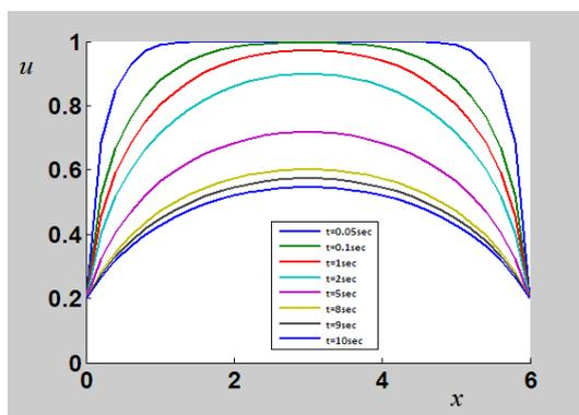
Fig. 2 Moisture content at several time for two dimensional case
