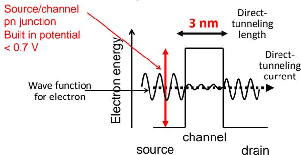
Even at  $L_g < 3 \text{ nm}$ , MOSFETs operate, but with huge leakage
