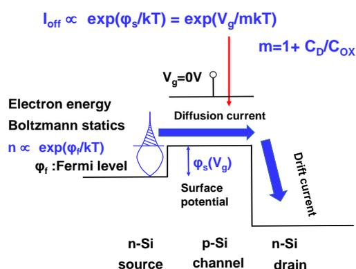
**Fig. 3** Subthreshold leakage current
