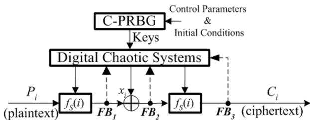
Figure 1: The encryption procedure
