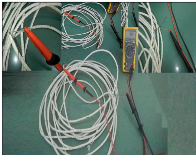
Fig.4 Thermal resistance long 20 meters that used to connection with device to test the Fault breaker.
