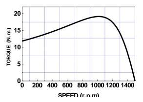
Fig.2. Torque/speed characteristics at constant parameters
