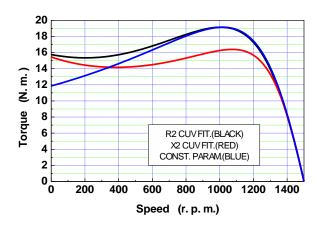
Fig.7. Torque / Speed relationship for different approaches
