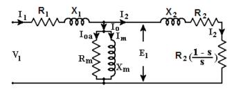
Fig.1. Equivalent circuit of three-phase induction motor
