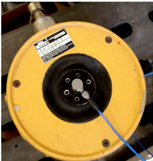
Fig. 1 ICP accelerometer fixed on the shaker
