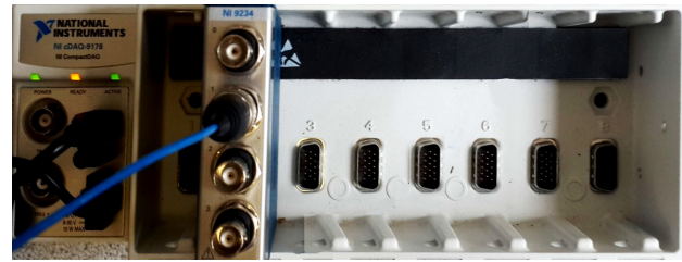
Fig. 2 NI cDAQ-9178 chassis with NI 9234 c-series module
