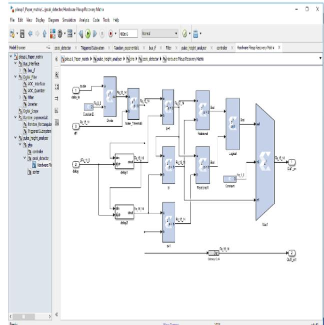
Fig. 2a: Matlab and Xilinx blocks for the hardware implementation of pileup recovery
