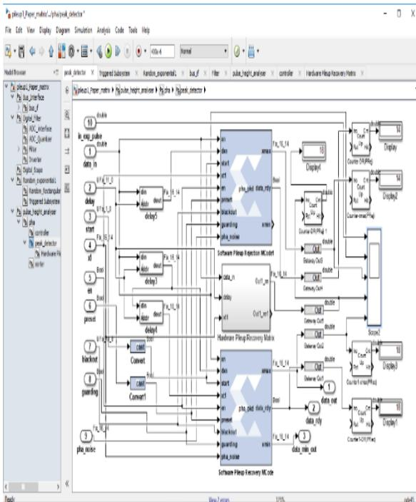
Fig. 2b: Simulation subsystems for pileup detection and rejection, hardware and software implementation of pileup detection and recovery
