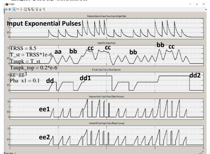
Fig. 3b: Pileup detection algorithms and output signals – Severe pileup situation
