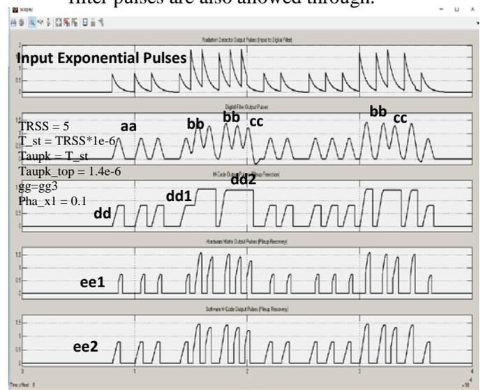
Fig. 3a: Pileup detection algorithms and output signals – Light pileup situation
