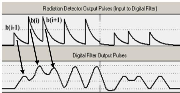
Figure 1: Pileup situation and response of a digital filter
