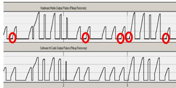
Fig. 4: Spurious detections by the detection blocks in the form of noise
