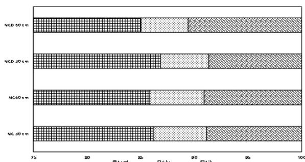
Fig.4. Soil particle size measured as percentage contribution of sand, clay and silt at mangrove forest in the non-disturbed site (NC) and the disturbed site (NCD) at 30 and 60 cm depth.
