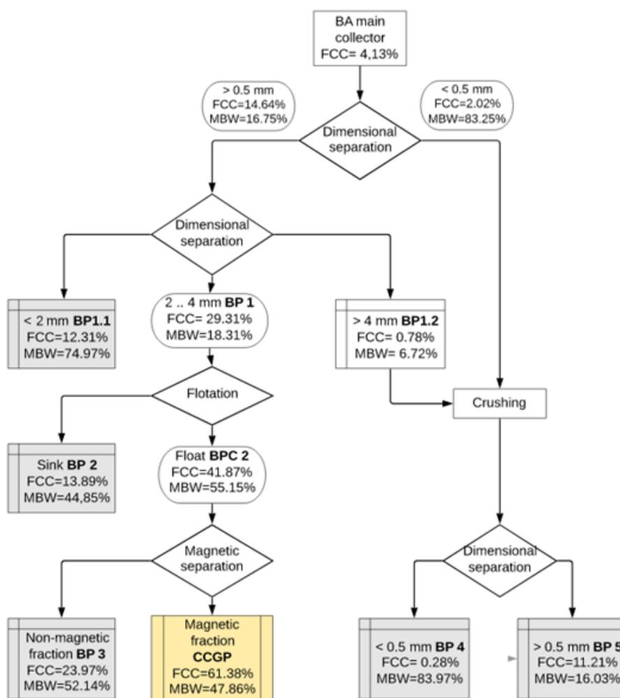
Figure 2. Overall process flow for complete BA recycling
