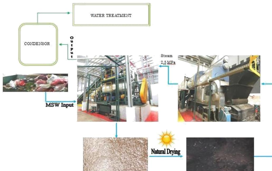
**Fig. 1.** Operating principle of HTT in Indonesia
