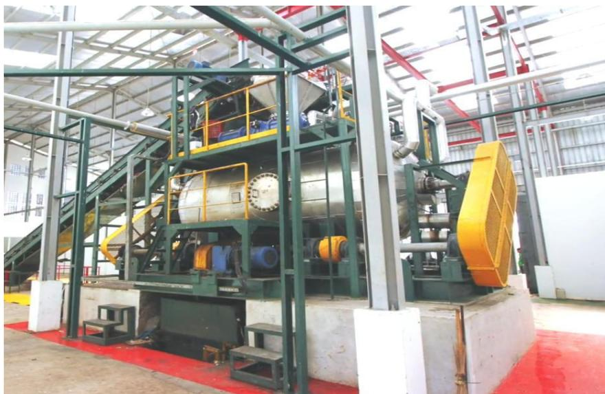
**Fig.2.** The reactor for the hydrothermal treatment installed in Tangerang, Indonesia
