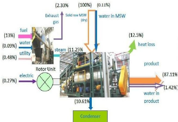
**Fig. 5.** Energy balance with 30 min. holding time
