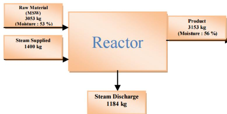
**Figure 4.** Mass balance with 45 min. holding time
