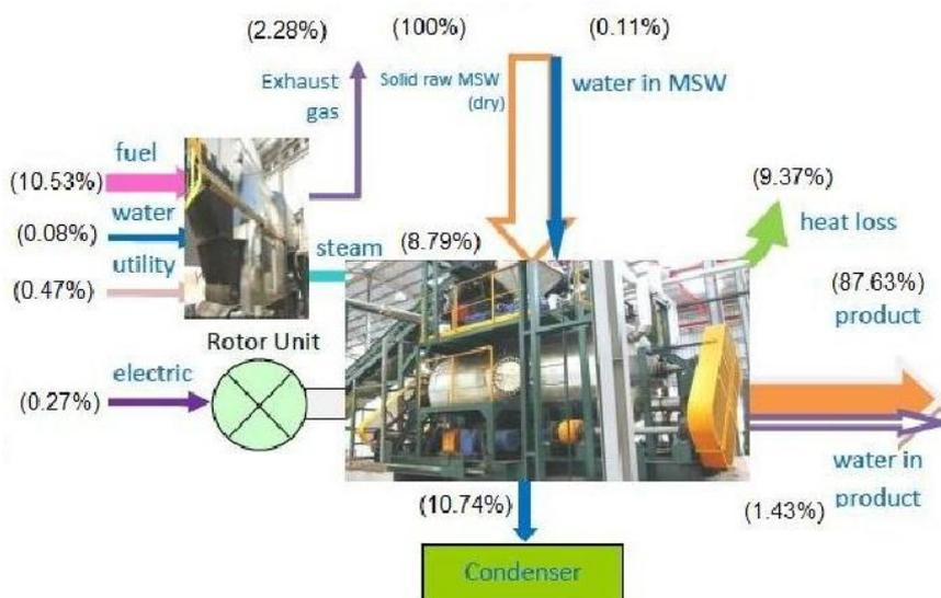
**Fig. 6.** Energy balance with 45 min. holding time
