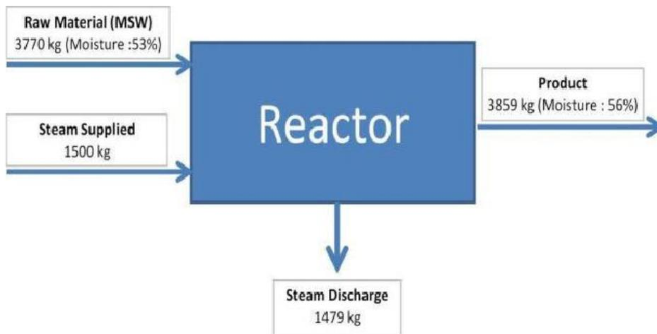
**Fig 3.** Mass balance with 30 min. holding time
