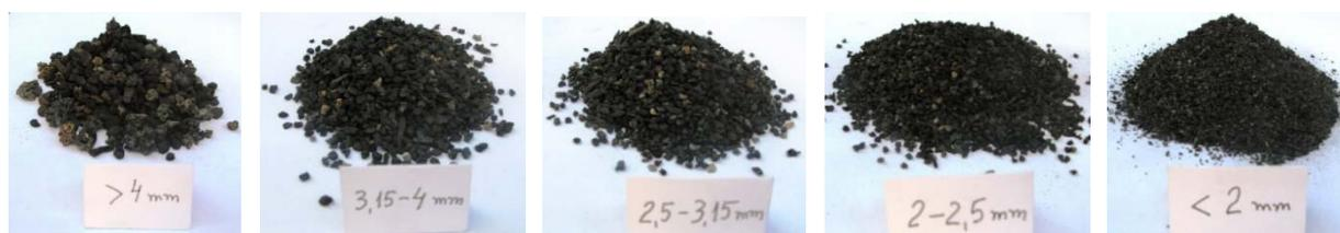
Figure 1. Heavy ash size fractions
