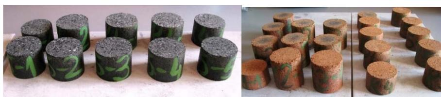
Figure 2. Test specimens (a – after casting, b – after drying and calcination)
