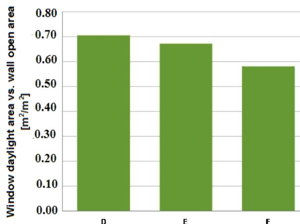
**Fig. 4** Ratio: daylight surface of the window glass compared with corresponding surface opening area in the wall [m<sup>2</sup>/m<sup>2</sup>].
