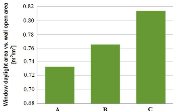
**Fig. 2** Ratio: daylight surface of the window glass compared with corresponding surface opening area in the wall [m<sup>2</sup>/m<sup>2</sup>]
